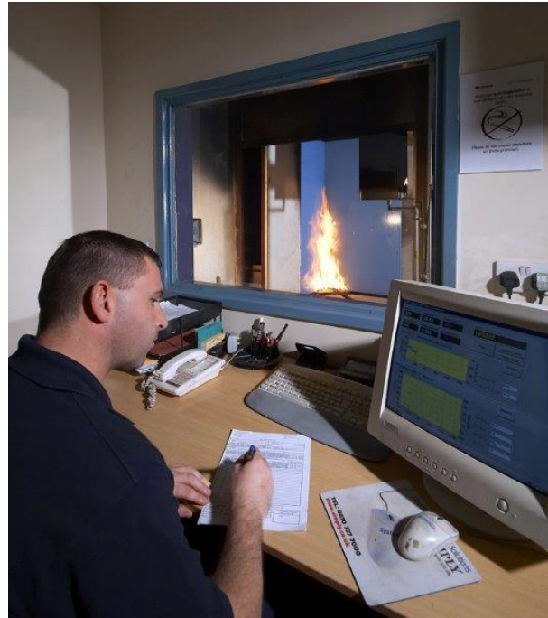
Figure 41: EN 13823 SBI test
