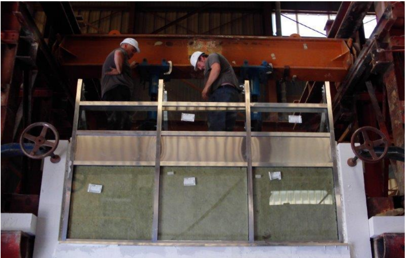
Figure 45: EN 1364-4 Curtain wall (part configuration) being prepared for fire testing
