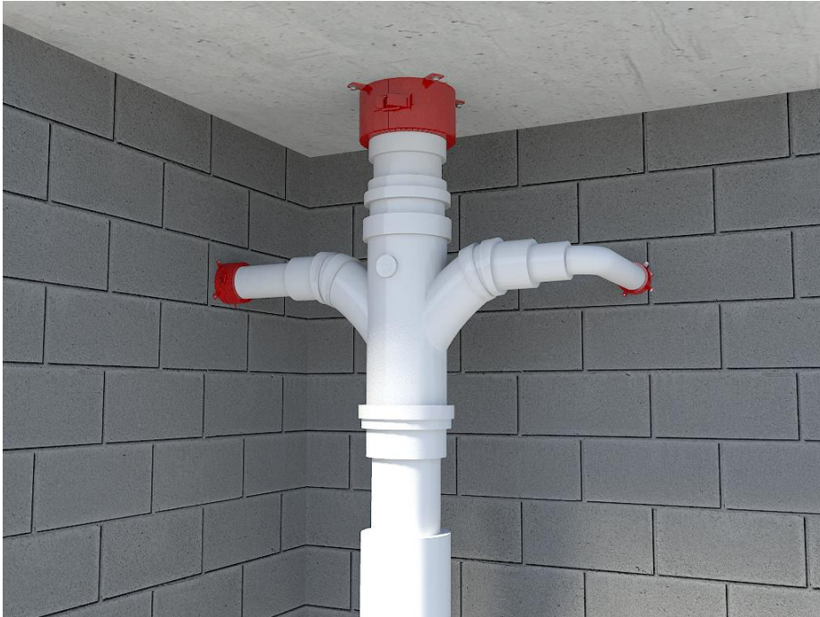
Figure 17: Pipe collar used at soffit of concrete floor and against masonry walls
