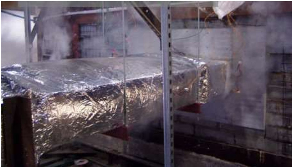
Figure 13: fire resisting duct under test
