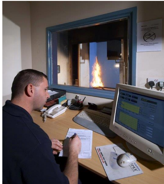
Figure 12: EN 13823 SBI test
