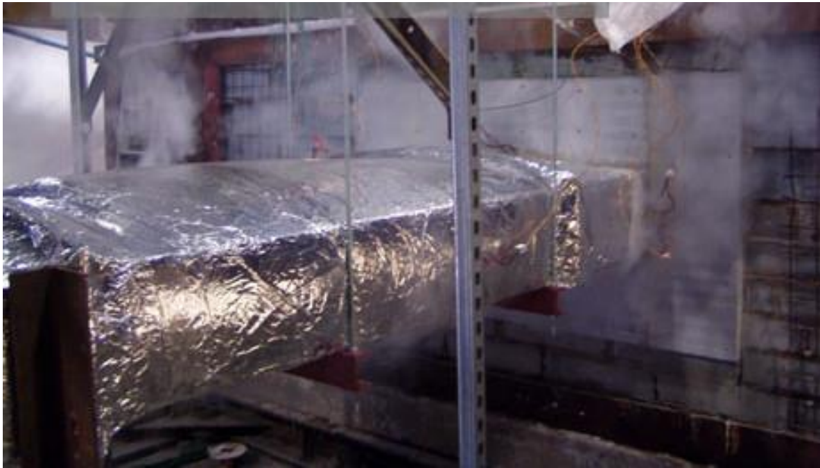
Figure 13: fire resisting duct under test
